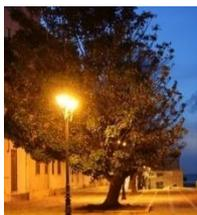
**High Pressure Sodium (HPS/SOx)**. Mainly used for streetlighting.
